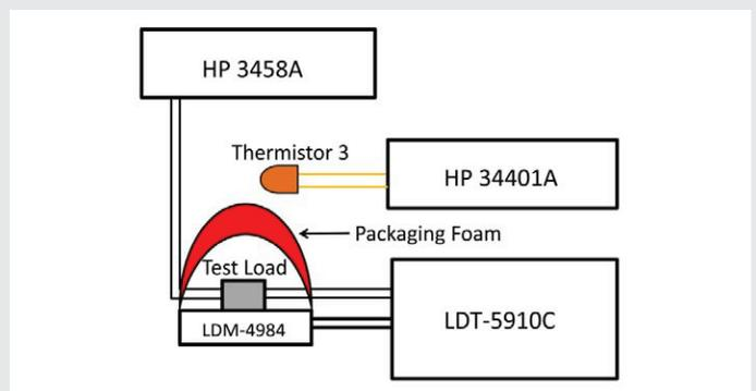
Figure 2: The temperature stability test setup.
